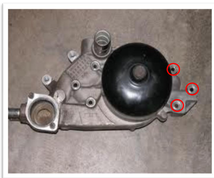
Vehicle requires LS1 style RH water pipe pump
