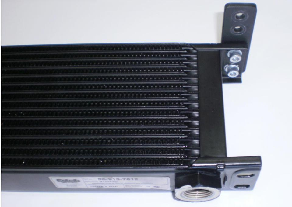
4. Assemble the two adaptor fittings into the oil cooler ensuring that the 'O' rings have been lightly lubricated with some engine oil. Note; Ensure that the hex fitting on the oil cooler is held with a spanner when tightening the fitting, no warranty given on twisted oil cooler fittings.
