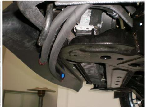
9. Connect the oil cooler lines to the adaptor manifold with the top (90 degree line) tightened prior to mounting. Fit the oil cooler adaptor manifold to the sump where the blanking cap was fitted. Ensure that the two small 'O' rings are fitted to the manifold. Connect the straight line and ensure everything is tight.
