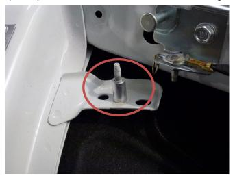
Place air box assembly into vehicle
