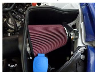
Place washer and M6 nut supplied on the mounting stud and tighten, also fit and tighten M6 cap screw supplied on the lower mounting tag.
