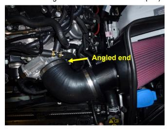
Once elbow is fitted place hose clamps in position and tighten. Insert connector to the MAF and connect the PCV hose on the fitting on the air filter adaptor, note hose routing.
