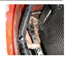
Check to ensure that the oil cooler has clearance from the low temp radiator.
