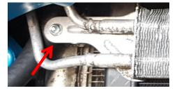
Mount the pump to the sheet metal below the LH rail using the supplied bracket as per image on the RH side (Note smaller pump shown in image).
