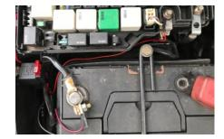
Mount the relay to the apron of the vehicle as per image shown. Feed the loom down to the pump and connect the pump.
