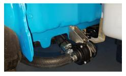
o Route the intercooler outlet to the inlet of the pump.
