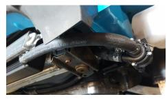
Route the intercooler lines from the pump outlet to the rear intercooler fittings connecting to the Y piece that splits the hoses.
