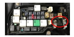
Lift the top section of the box up by releasing the retaining tabs around the outside perimeter of the fuse box.
