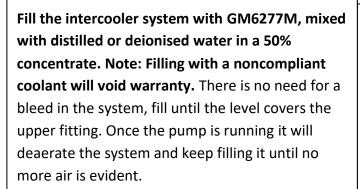
The vehicle should start with the standard file, run the engine to confirm no leaks in the intercooler system and fuel line.
