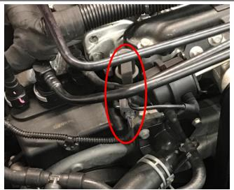
Remove the supercharger drive belt, 15mm AF.
