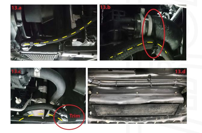
14. The radiator channel will also need to be folded away from the hose at both the left and right side to provide clearance away from sharp edges as per image below. (RHS shown)
