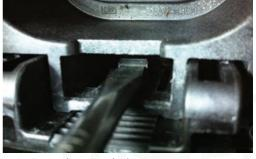
2.c. Remove the two lower sections of the mounts. Remove the 2 M6 bolts.Note: Retain the bolts to use with the OTR specific radiator brackets.2.d. Use needle nose pliers or similar to compress the clips on the loom and push them through the lower section of the radiator mount. There are 2 clips for each mount.
