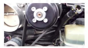
11.f. Install the throttle body into the rubber boot at the back of the OTR. Fit a 91-114mm hose clamp to back of OTR/boot but do not tighten.
