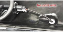
24.a. Insert the 90 degree quick connect fitting into the rubber boot on the OTR. Ensure the locating bead locks the fitting into position.
