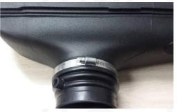
21.a. Install the throttle body into the rubber boot at the back of the OTR.
