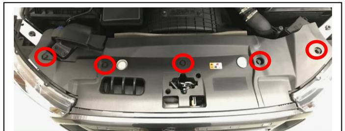
To assist in getting your hand down to release the spring clips that lock the charge air intercooler hoses to the intercooler on the left hand side, it is advisable to unscrew this module so that it can be pushed aside.
