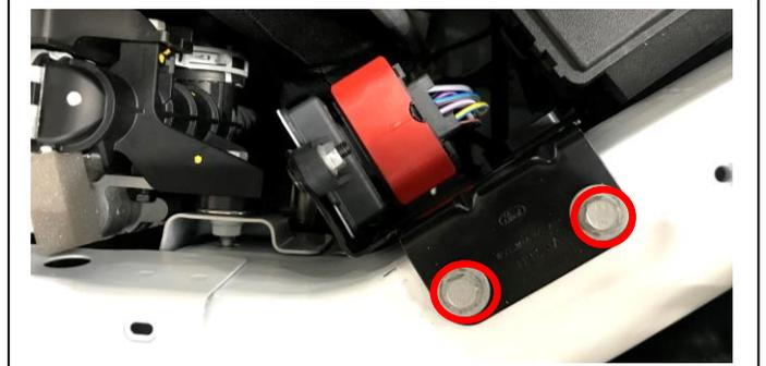
Unscrew the upper grill screw on each side. Now unscrew and remove the intermediate mounting screw just inboard of the head lamp.
