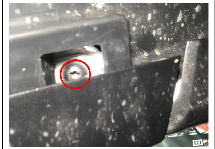
Undo and remove the 3 screws that secure the flare to the front bar cover. The wheel liner should now be free to move out from between the flare and the front bar cover.
