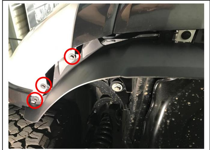
Undo and remove the vertical screw that joins the front bar cover to the fender.
