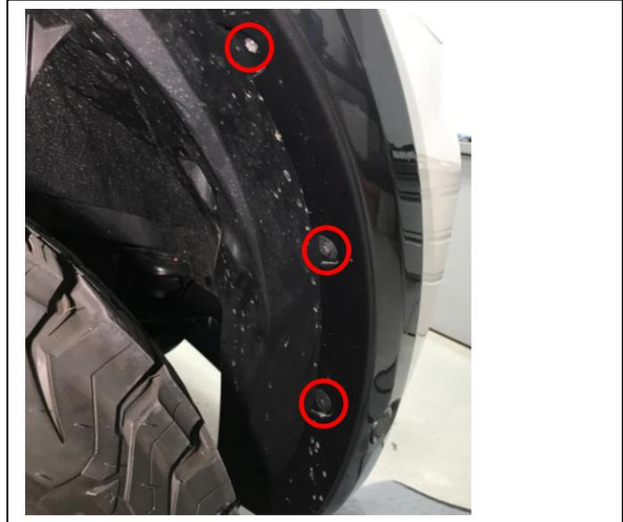
The side of the bar cover now needs to be popped out of the clips securing it to the fender and under the head lamp. Gently pull the bar cover away from the fender outward. The bar cover can now be removed so that access to disconnecting the driving lights and the bar cover harness on the LH side can be completed and bar cover placed aside.
