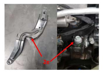
f) Remove the Fuel purge solenoid bracket, quick connect line and loom plug.
