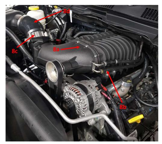
e) Push the Fuel Purge Solenoid onto the bracket on the RHS of the Supercharger.
