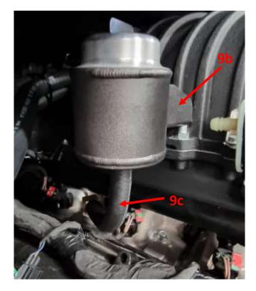
d) Using the supplied 3/8" x 800 long PCV hose, connect the top barb of the PCV housing to the Top barb on the supercharger inlet cover. Trim to length as required.
