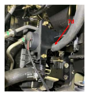
e) Connect the 1000mm long ¾" hose between the bottom port of the coolant reservoir bottle and the top port of the intercooler reservoir to complete the circuit.
