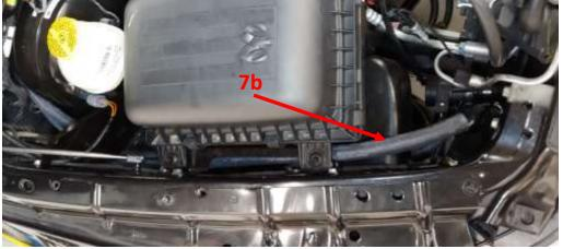
c) Connect the 2x intercooler outlet hoses to the reservoir.
