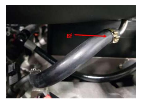
g) Using the supplied <sup>3</sup>/<sub>4</sub>" plastic hose joiner, connect the PCV vent hose (coming from the oil filler tube) to the inlet boot.
