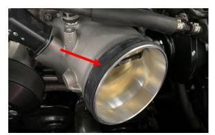
Feed the slotted end of the carbon duct through the hole from the inside of the airbox, ensuring that the rubber seal stays in place around the airbox hole. Rotate the duct roughly into its correct orientation.
