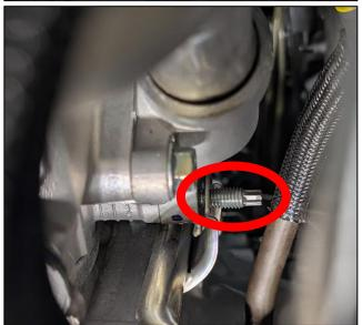
cc. Install the provided bracket between the block and the heater line reusing the bolt into the block and the included M6x12 socket head cap screw and M6 flanged nut through the bracket.
