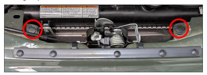
b. Undo the 2 clips at the bottom of the grill with a Phillips head screwdriver.
