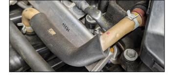
m. Remove fuel rail from the engine, ensuring that the tips do not fall off the injectors into the engine.
