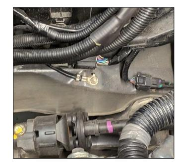
d. Install pump mount reusing existing hardware ensuring that the earth lead is reattached. If in step 4b, there was no harness bracket to remove, install the supplied M6x20 socket head flange screw.
