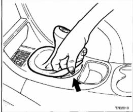
Inside the vehicle, remove the gearshift knob by with the fingers of one hand hooked under the edge of the gearshift lever boot as shown, carefully release each of the 8 plastic retainers and free the gearshift lever boot from the console cap. **NOTE:** The gearshift lever knob and console boot are manufactured as a single component. Do not attempt to remove the gearshift lever knob separately to the boot.
