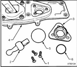
Remove the front pivot pin from the bridging piece. These pins are an interference fit into the bridging piece so care must be taken not to damage the pin as it is used for reassembly.
