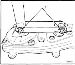
Inside the vehicle, pull back the remote shifter lever boot and tuck back under rear of console to gain access to the top of the gearbox. Remove three screws from plastic dust cover, then remove four remote shifter to gearbox mounting socket head bolts, and remove remote shifter from vehicle.
