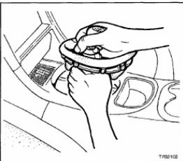
Lift the gearshift lever boot enough to enable a firm grasp to be made on the gearshift lever with the left hand, then grasp the gearshift knob with the right. While rocking the knob sideways, with an upward force applied, dislodge the knob retaining claws from the lever. Remove the gearshift lever knob and boot assembly from the gearshift lever.
