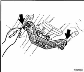
Slowly and carefully raise the transmission, then refit the four engine rear cross-member to side frame attaching bolts, ensuring correct alignment with the original scribed lines. Refit the four exhaust to catalytic converter bolts.
