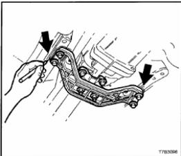
From under the vehicle, remove the four bolts securing the remote shift lever boot to the floor pan. Scribe around each of the transmission support cross-member mounting points to the vehicle under-body, to provide an alignment reference for reassembly.
