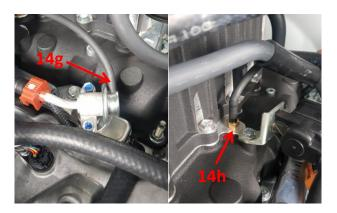
h) Connect the other end of the  $\emptyset$ 4.0mm hose to the barb fitting on the LHS of the supercharger manifold, adjacent to the fuel purge valve.
