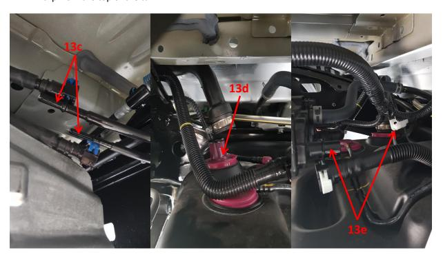
f) Dis-connect the fuel vent line at the filler neck.
