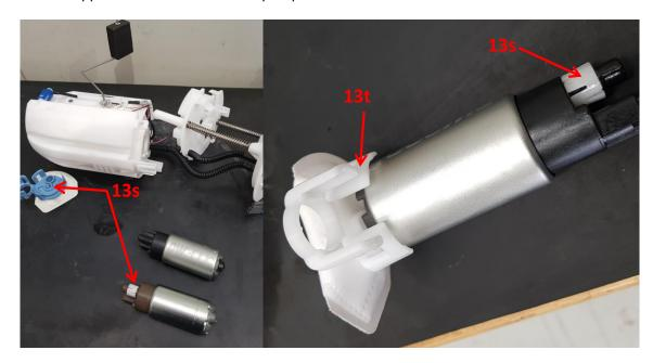
u) Inspect the O-ring in the fuel pump housing. Replace with a new supplied O-ring of the same dimensions if it is worn or damaged.
