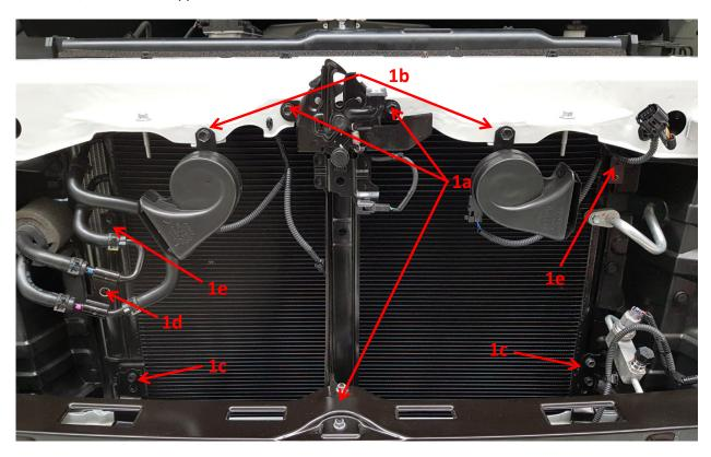
f) Swap top A/C condenser bracket rubber bushes to Harrop radiator. Mount the Intercooler radiator onto the original pins on the top cross-member (adjacent to the horns).
