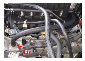
n) Using the remaining 750mm long ½" vacuum hose, connect between the LH facing branch of the T-piece and the LH Rocker cover.
