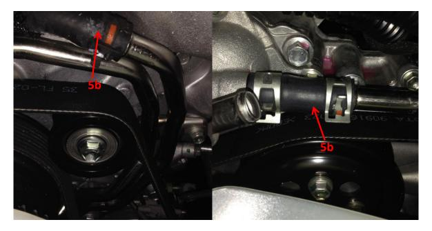
c) Remove the Toyota elbow hoses at the oil cooler under the LH front of the vehicle.
