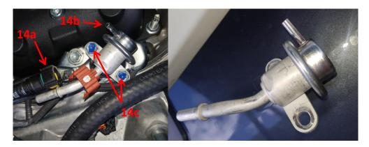
c) Un-screw the 2x M6 bolts that secure the regulator to the fuel-rail and remove the regulator.
