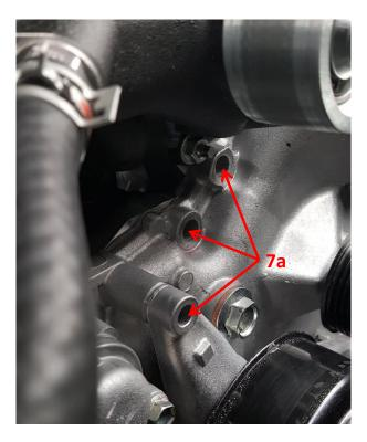
b) Install the Harrop supercharger idler bracket using the supplied bolts.
