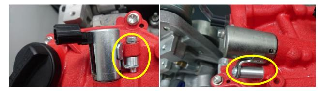
On the front valve cover remove the existing PCV valve and install the supplied 90 degree hose connection. Use Loctite 567 on the thread to seal off into the valve cover. Screw the main fitting in until it becomes tight and the openings align with the valve cover. Install the tail piece fitting on the opening pointing towards the left hand side of the car using Loctite 567 on the thread and in the other end screw in the plug.
