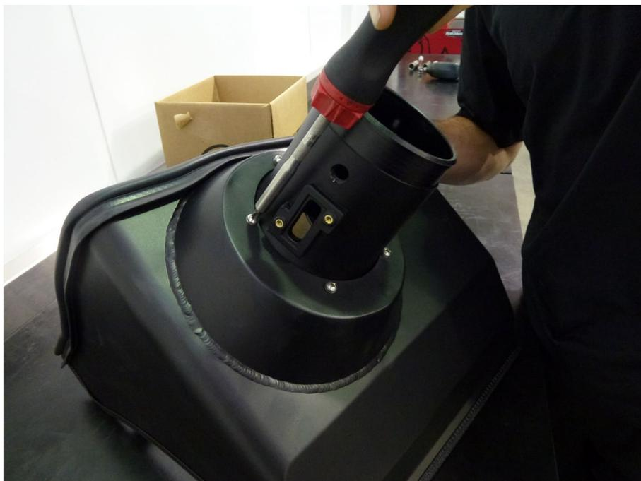
Place MAF card into slot and screw into place
