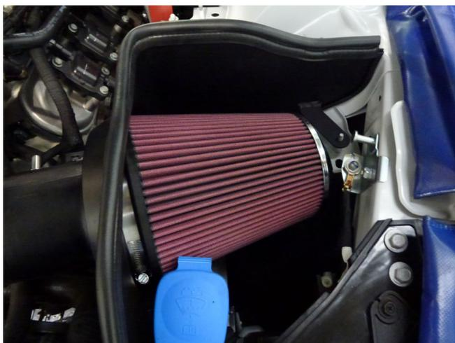
Place washer and M6 nut supplied on the mounting stud and tighten, also fit and tighten M6 cap screw supplied on the lower mounting tag.
