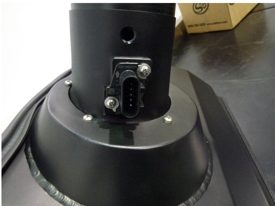
Screw in PCV hose adaptor provided into air filter adaptor
