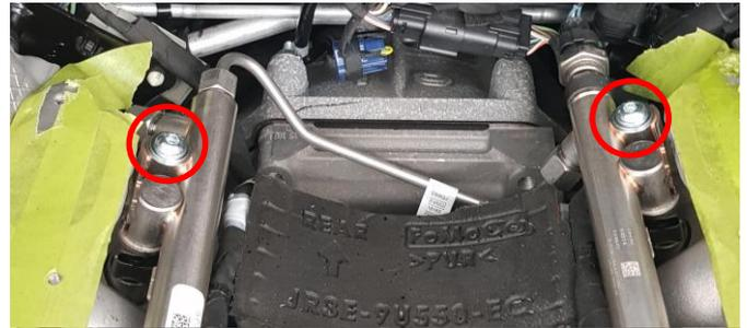
To install the manifold the upper lid needs to be removed from the supercharger to enable the inner 4 screws to be installed. Remove the M6 screws and the 1 M8 securing the by-pass and remove lid assembly. Ensure that the TMAP sensor loom is attached to the manifold and the fuel line connection points are tight.
