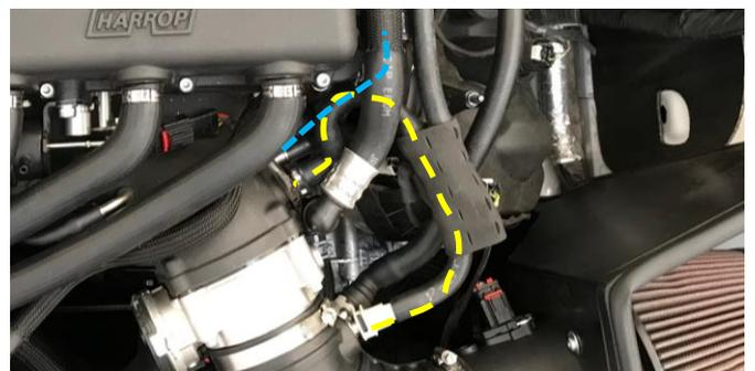
Connect the LH valve cover breather to the lower fitting of the clean air intake tube.
