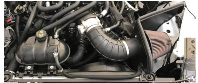
Install this assembly into the engine bay, main fixing point is on the lower left hand rail.
