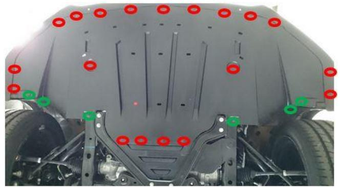
On the MY18 vehicles the air seals have been upgraded and there is an additional seal to be removed from the lower side of the radiator air outlet. Remove the outer two screws from the cross tie bars.
