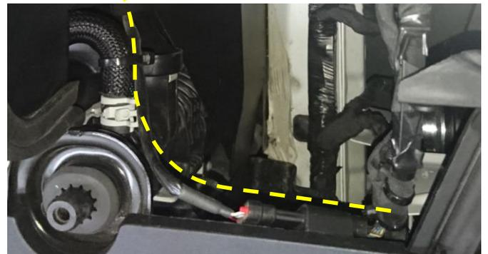
Connect the fuel purge hose as per blue line to the rear fitting on the inlet of the supercharger and the reworked booster assembly as per yellow line, front fitting on the supercharger and the upper fitting on the clean air tube.
