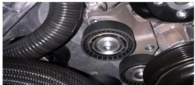
Install the supercharger drive belt, note the belt run in green on the image, you will need a 3/8 square drive brace for the tensioner.
