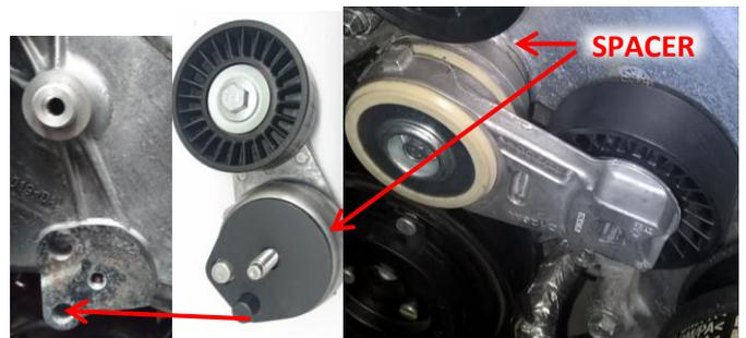
Fit the new idler pulley supplied to the boss above the just fitted tensioner using the supplied bolt and washer, torque the bolt to **24Nm**
