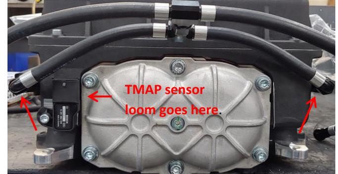
For MY18 vehicles transfer the factory intake port seals from the NA manifold to the supercharger manifold. MY15-17 fit the new MY18 seals supplied. For MY18 vehicles with the DI system, remove the original fuel pressure/temp sensor and install into the LH fuel rail, torque to **6Nm** and then tighten another **25** degrees. Install the 4 supplied 'O' rings in the bottom sealing face of the manifold for the 4 inner mounting screws. See image right.
