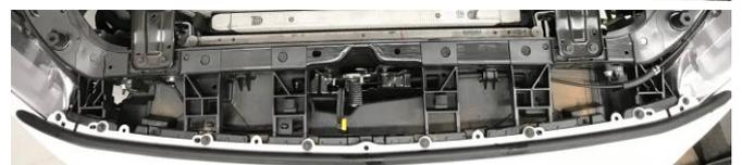
Remove the under tray from the vehicle. There are **19 screws** and **6 scrivets**.
