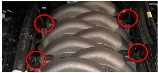
Disconnect the injectors and undo the 10x8mm manifold retaining screws. Note some of these also hold the fuel rails in place which do not need to be separated from the manifold for MY15-17. The injectors are reused for the MY18 vehicles so if working on MY18 vehicle remove the injectors from the rail/manifold and place aside. MY18 vehicles also reuse the fuel pressure sensor, disconnect this now.
