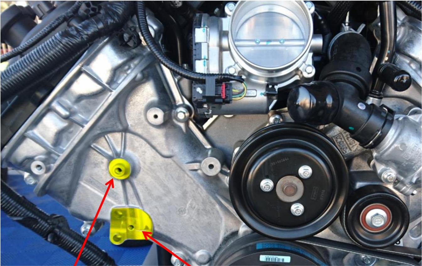
This boss has been machined and the hole has been threaded.
