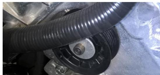
Remove the water pump pulley so that the supplied idler bracket and pulley assembly can be mounted. Remove one screw from the water pump that is at the 10 O'clock position, remove the two timing cover bolts where the new idler bracket will mount. Mount the assembly and torque the bolts to **24Nm**.
