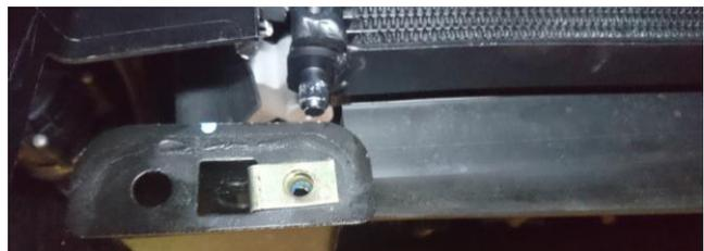
Install the lower mounting plates with the supplied rubber isolators as per image using the supplied M6 screws.
