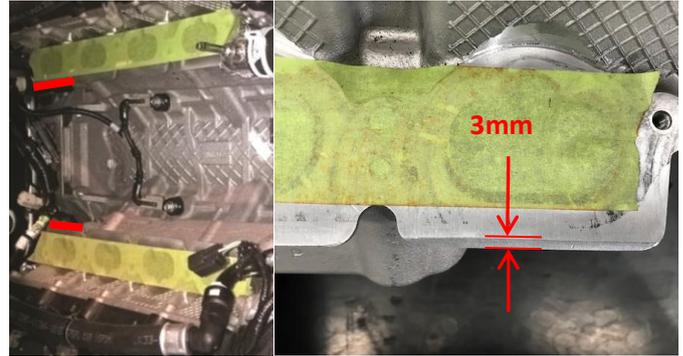
For the MY18, DI engine you will need to remove the rear DI rail mounting bolts and replace them with the 2 button head screws supplied. Use low strength thread locker Loctite 243. Torque to **24Nm**.
