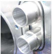
Reassemble the throttle body adaptor to the supercharger manifold. Torque the 7 M6 socket head cap screws to 11Nm
