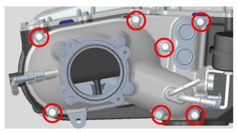
Once the inlet adaptor is on you will now need to pack in 2 beads of silicone, Loctite SI 587 flange sealant as per images below, it needs to go down about 10mm. Note this is an RTV and will need time to cure.
