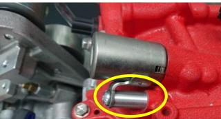
On the front valve cover remove the existing PCV valve and install the supplied 90 degree hose connection. Use Loctite 567 on the thread to seal off into the valve cover. Screw the main fitting in until it becomes tight and the openings align with the valve cover. Install the tail piece fitting on the opening pointing towards the left hand side of the car using Loctite 567 on the thread and in the other end screw in the plug.
