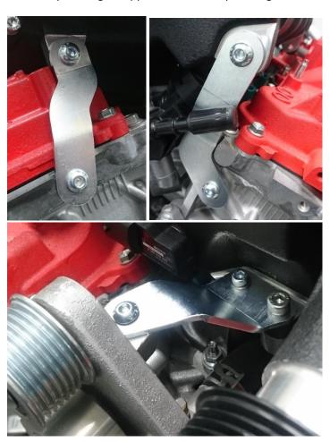
Reinstall the intercooler core into the manifold making sure there is no foreign material inside any ports or manifold, use Loctite 243 on the screws as a thread locker. Torque these screws to 11Nm.
