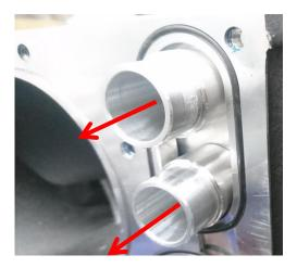
Remove the upper manifold lid, 20 x M6 socket head cap screws. Remove the 4 screws from the intercooler, now placing some fingers inside the area where the spigots were lift the core up slightly enough to get a grip on the lid side to remove the core from the manifold.
