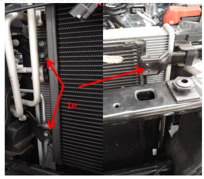
f) Secure bottom LH corner of intercooler using supplied bracket, 14562, and supplied fasteners to attach to the supercooling bottle of the air conditioning system. Use a small amount of silicone to secure bracket to bottle before tightening fasteners.
