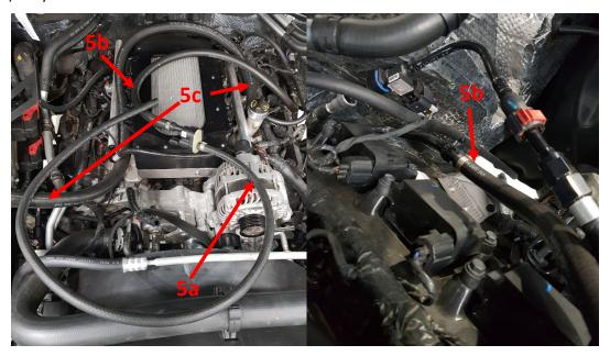
e) Using a tube cutter, shorten the brake booster hard-line as shown below
