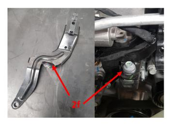
g) Remove the Fuel purge solenoid bracket, quick connect line and loom plug.
