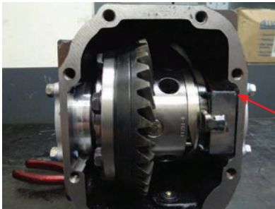
Clearance around the tab
